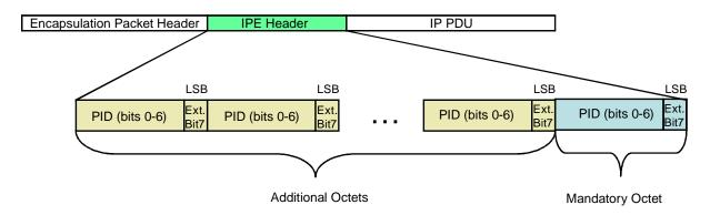
Figure A-2: IPE Header Format and Placement
