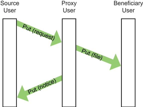
**Figure 2-6: Proxy Put Operations, Sequence of Events**
